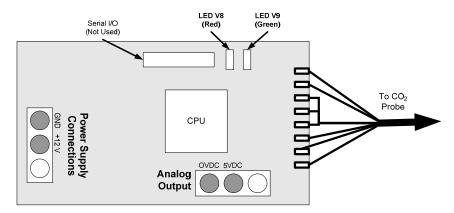
Figure 12-13: Location of Diagnostic LEDs onCO<sub>2</sub> Sensor PCA
